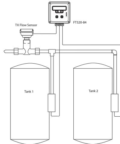
**Connections for Alternating Tanks**
